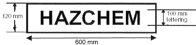
Figure 13.1 Form and dimensions of outer warning placard
